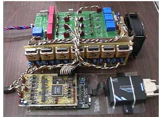
Fig. 9 230V, 3 kVA laboratory prototype matrix converter
